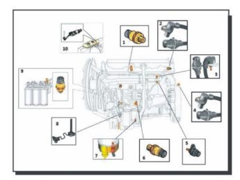
The **Electronic Management System** continuously monitors and gathers date from 10 different sensors in the engine and adjusts the fuel supply and injection timing at lightning speed. This maximized fuel efficiency and engine output at any given time. It also enables precise integration of the engine with the machine that it powers and provides enhanced engine protection.
